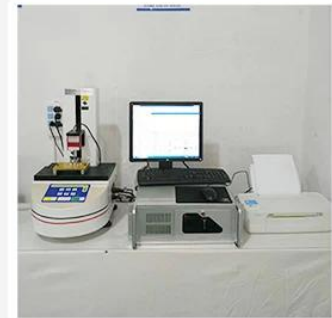
3. Load Curve Meter
