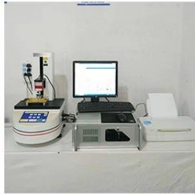
3. Load Curve Meter
