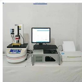
3. Load Curve Meter
