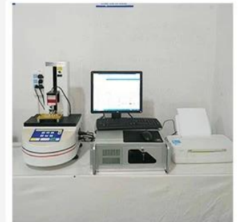
3. Load Curve Meter
