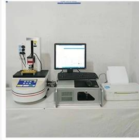
3. Load Curve Meter
