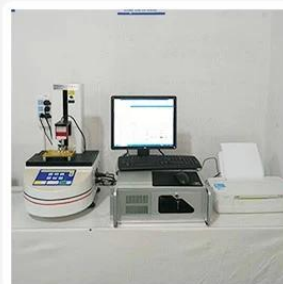
3. Load Curve Meter
