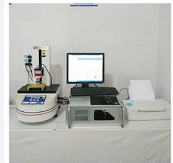
3. Load Curve Meter
