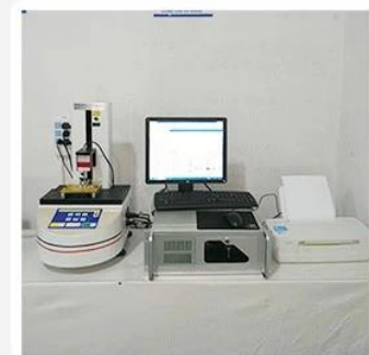
3. Load Curve Meter
