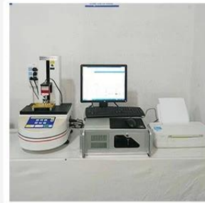
3. Load Curve Meter
