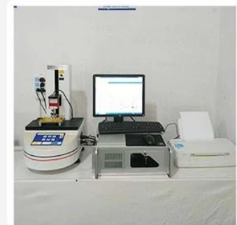
3. Load Curve Meter
