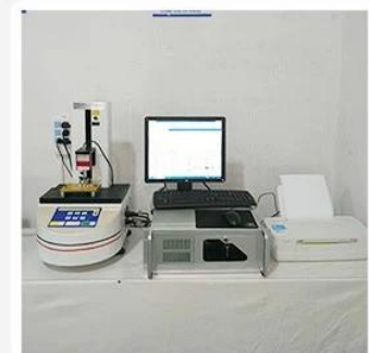
3. Load Curve Meter
