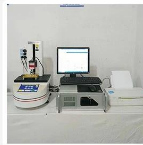
3. Load Curve Meter
