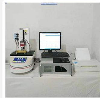
3. Load Curve Meter
