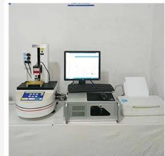
3. Load Curve Meter
