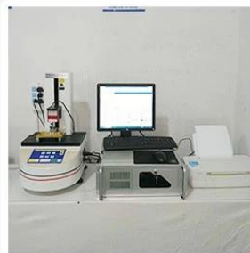
3. Load Curve Meter
