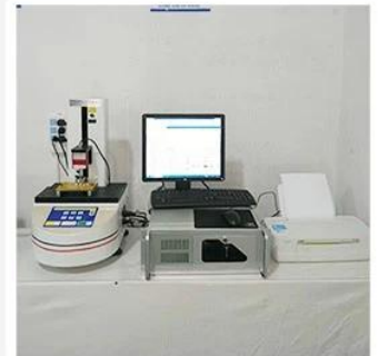
3. Load Curve Meter
