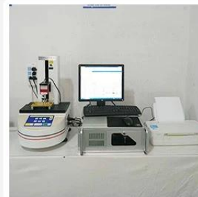
3. Load Curve Meter
