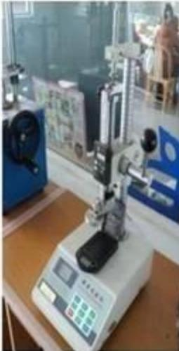
A white and blue machine with a vertical column and a horizontal arm, used for testing the spring constant of coils.                      |
