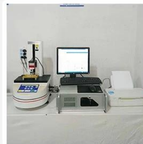
3. Load Curve Meter
