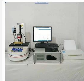
3. Load Curve Meter
