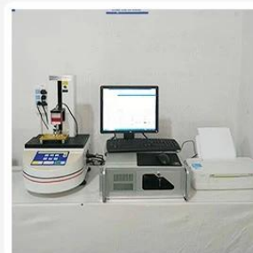
3. Load Curve Meter
