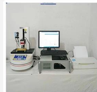
3. Load Curve Meter
