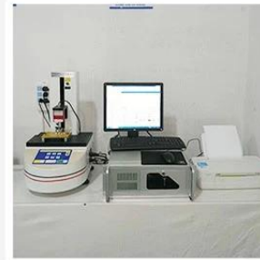
3. Load Curve Meter
