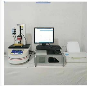
3. Load Curve Meter
