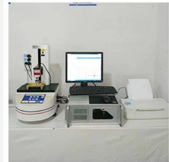
3. Load Curve Meter
