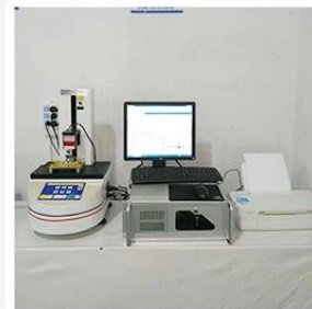
3. Load Curve Meter
