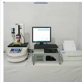
3. Load Curve Meter
