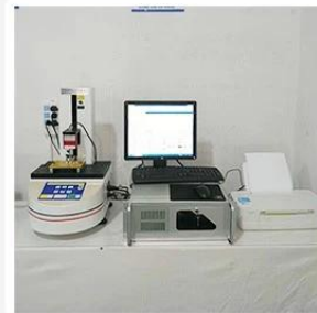
3. Load Curve Meter
