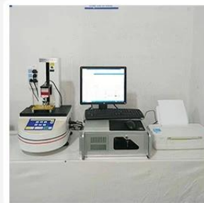
3. Load Curve Meter
