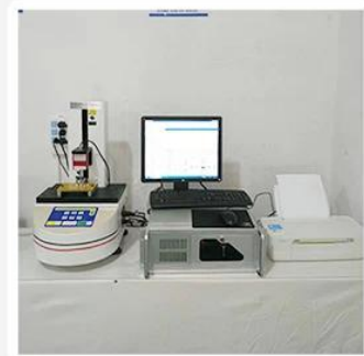
3. Load Curve Meter
