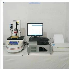
3. Load Curve Meter
