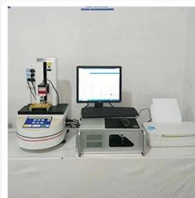
3. Load Curve Meter
