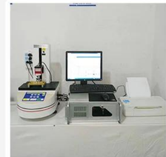
3. Load Curve Meter
