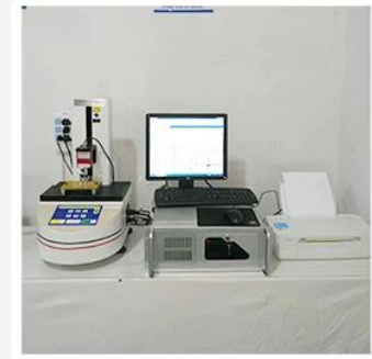
3. Load Curve Meter
