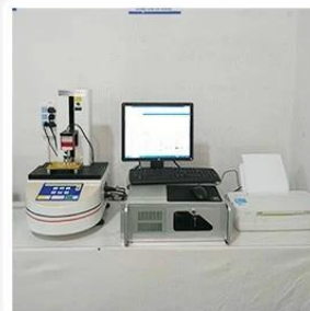
3. Load Curve Meter
