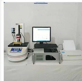
3. Load Curve Meter
