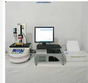
3. Load Curve Meter
