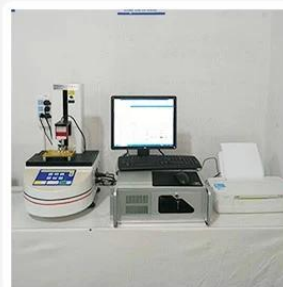
3. Load Curve Meter
