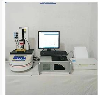
3. Load Curve Meter
