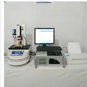
3. Load Curve Meter
