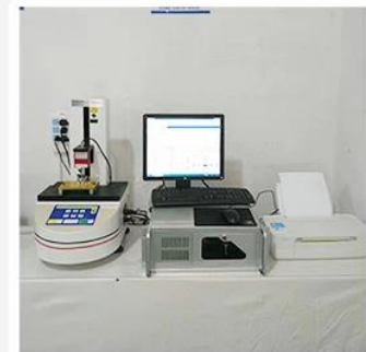
3. Load Curve Meter
