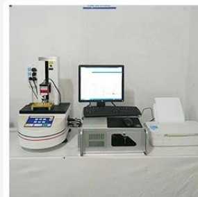
3. Load Curve Meter
