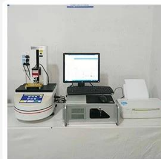
3. Load Curve Meter
