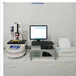
3. Load Curve Meter
