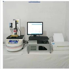
3. Load Curve Meter
