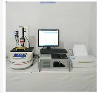
3. Load Curve Meter
