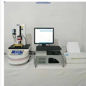
3. Load Curve Meter
