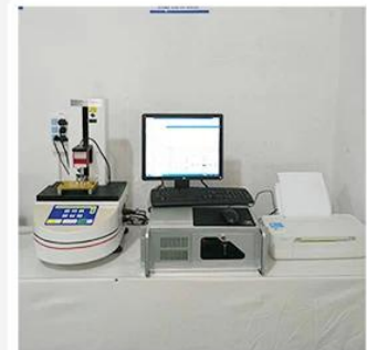
3. Load Curve Meter
