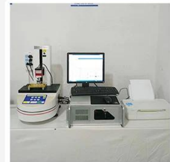
3. Load Curve Meter
