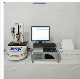
3. Load Curve Meter
